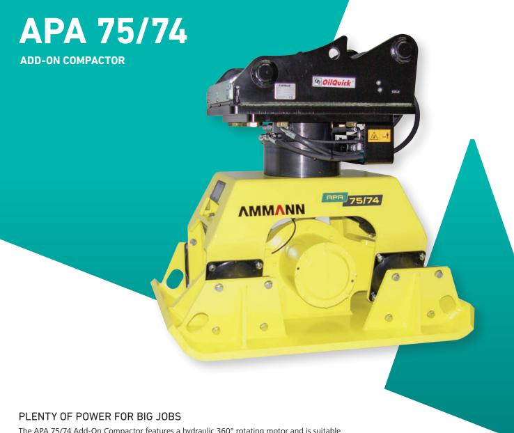
The APA 75/74 Add-On Compactor features a hydraulic 360° rotating motor and is suitable for excavators in the 12- to 25-tonne class. This makes it ideal for use in widely varying site conditions including trenches and other confined working areas, and also in more open spaces where productivity is required. Depending on the excavator size, the APA 75/74 can reach a depth of up to one meter Fill depths of more than half a meter can be compacted.
